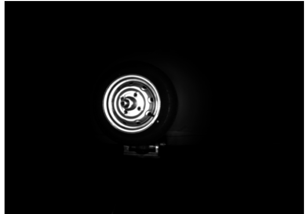
Fig. 10. Right camera rectified tilted wheel image
