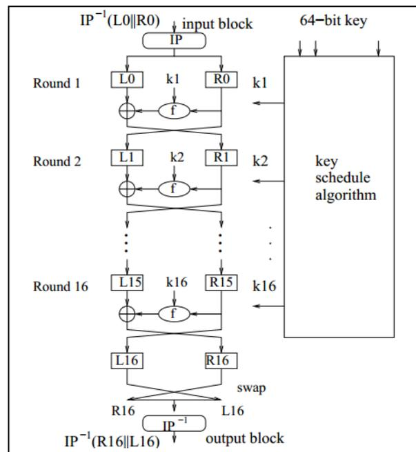
Figure 1. DES Encryption
