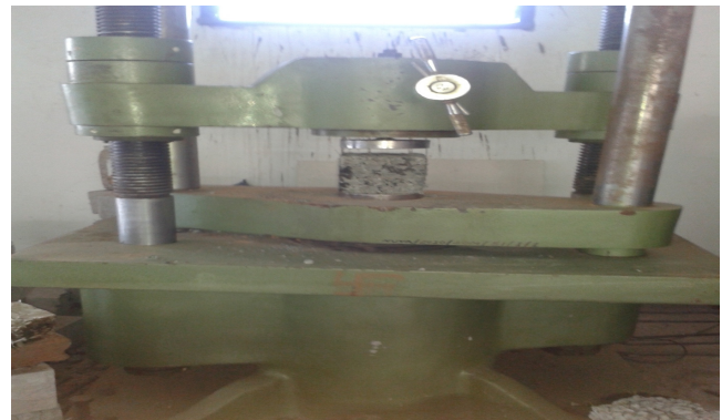
Fig. 12 Compressive Strength Machine (UTM)
