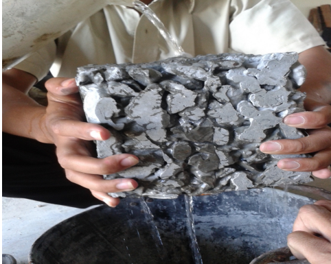
Fig. 13 Permeability testing of plain pervious concrete cube
