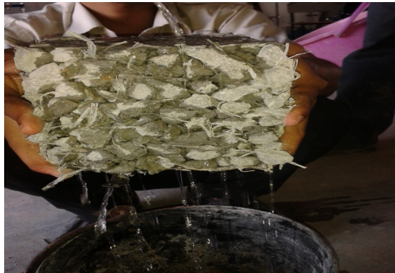
Fig. 14 Permeability testing of fibre mixed pervious concrete cubes
