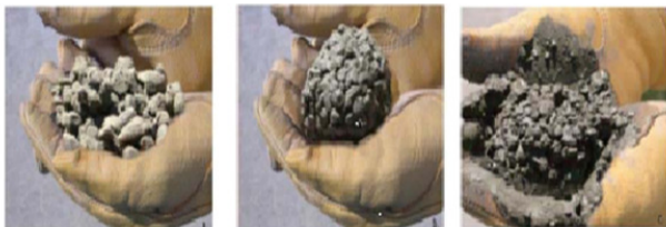
(A) Too little water (B) proper amount of water (C) too much water
