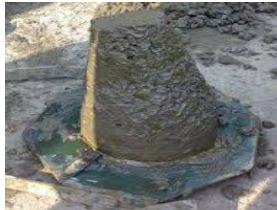
Fig. 11 Slump Cone Test
