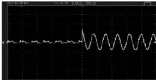
Fig. 17. Current of the resonance part during fault (current/div.: 5 A; time/div.:25 ms).
