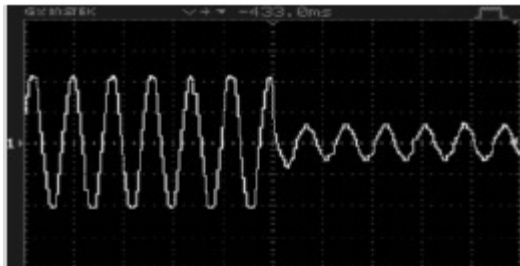
Fig. 18. PCC voltage without using the FCL (voltage/div.: 50 V; time/div.: 25 ms).
